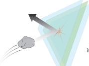
Optional laminated glass is a difficult-to-penetrate laminate layer between two panes of glass. Located on the interior side of the window, the laminated laver makes it very difficult for someone to force entry into your home through the window.
