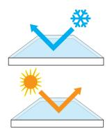
All 7700 windows help to lower energy costs because they feature Low E glass and Argon gas inside the insulating glass unit. Low E glass helps keep heated air inside during colder months and air-conditioned air inside during warmer months. Argon gas is a non-toxic gas that is heavier than air. By replacing the air inside the insulating glass unit with Argon, it adds higher insulating values and increases efficiency.
