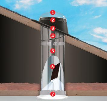
VELUX Sun Tunnel Skylights<sup>®</sup> fit between ceiling beams, allowing sunlight to travel from the roof to the space below uninhibited.
