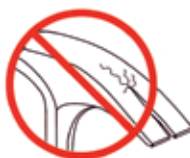
Crack in claw section
